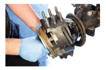
**STEP 9 - CHECK STEERING PRELOAD**
